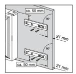
6. Place guide (Ha) on the inside part of the furniture door, up and down as shown in the figure and mark the position of external holes. After having drilled holes, fix the guide with the screws supplied.
